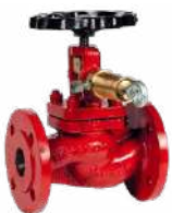
QUICK CLOSING GLOBE VALVES, DIN PN10/ PN16 FLANGED NODULAR CAST IRON BODY, STAINLESS STEEL TRIM, WITH LR CLASS CERTIFICATE
