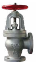
ANGLE VALVES, JIS 5K - WITH DNV-GL CLASS CERTIFICATE CAST STEEL BODY, STAINLESS STEEL TRIM, SCREW DOWN NON RETURN (SDNR)
