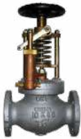
QUICK CLOSING GLOBE VALVES, DIN PN10/ PN16 FLANGED NODULAR CAST IRON BODY, STAINLESS STEEL TRIM, WITH LR CLASS CERTIFICATE
