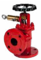
QUICK CLOSING ANGLE VALVES, DIN PN10/ PN16 FLANGED NODULAR CAST IRON BODY, STAINLESS STEEL TRIM, WITH LR CLASS CERTIFICATE
